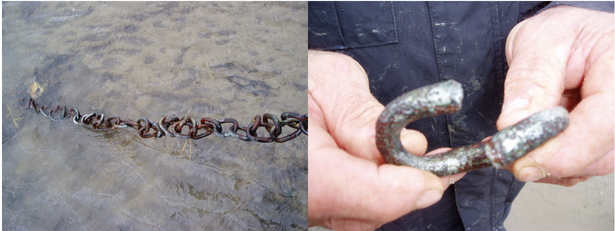
The riser chain attached to the root. The riser was even more twisted when first seen.
