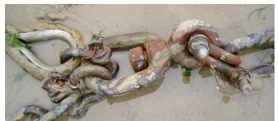
Oversized swivel allows two shackles (with bolts & nyloc nuts) to riser, & rope + chain pennants.
