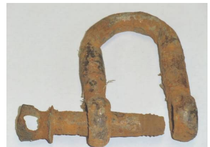
Cheap shackle after a season. Only mousing held the pin in.
